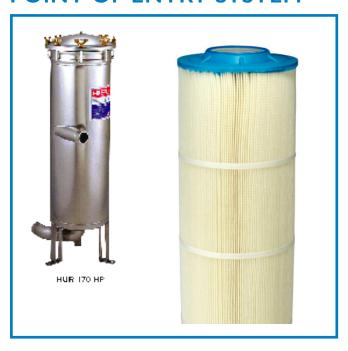
Our Point of Entry (POE) filter is the ultimate barrier for your water applications, including potable water, cooling systems, closed loops, and other applications. The 304SS housing six 20" clean in place 0.2 micron filters to allow for flow rates up to 30 GPM.
