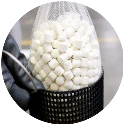
Pellets are placed into the pellet cage, which is then inserted in the feeder.
